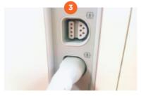
Connect the ANI MOC-9 module to one of three MOC-9 ports on Root
